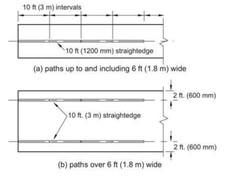
Fig. 1 Non-ramp pedestrian path flatness measurement for running slope
