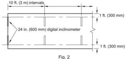
Non-ramp pedestrian path flatness measurement for cross slope
