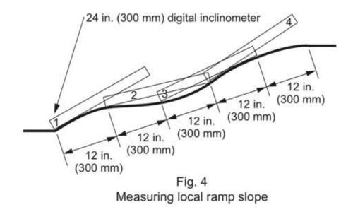
Measuring one - foot (300 mm) lengths allows for a reasonable check on local variation that can be accomplished easily and inexpensively with a 2 - ft digital inclinometer or other available instruments.
