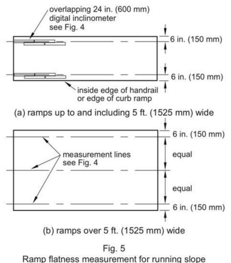
Ramp namess measurement for running slope
